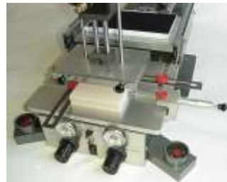
Inked stamp die contacts mount in exact location and with even pressure
